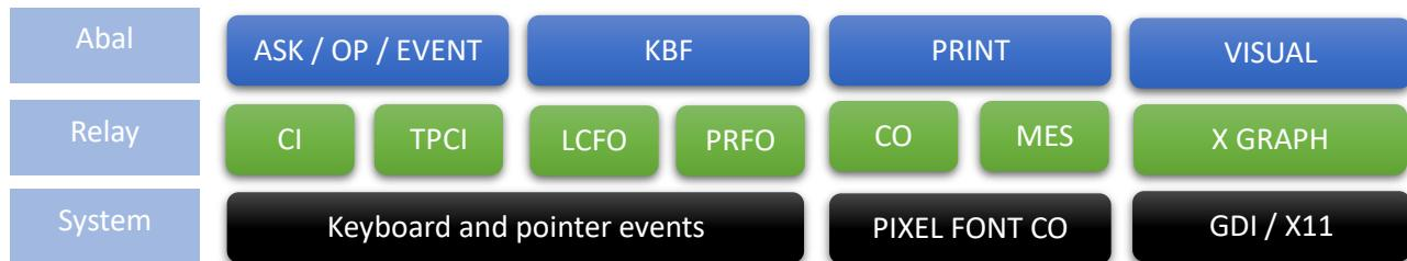
With the addition of the GIGO subsystem, an extra relay was added to provide the abstraction for the graphical operations. The other relays are overloaded and connected through to the graphical CI and CO emulation using the underlying PIXEL font management and operating keyboard and pointer device event management.
