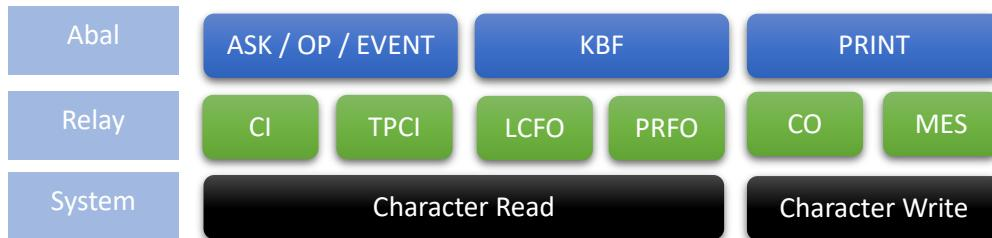
The CI, TPCI, LCFO, PRFO, CO, and MES relays provide a generic abstraction for the ABAL instructions to access the underlying terminal management, through the corresponding system dependent read and write calls. Since all PRINT output is directed through the CO and MES relays, the overloading of these relays can be performed by ABAL visualisation libraries, such asASFUN and VISUAL, facilitating the seamless integration of their enhanced windowing and graphical functionalities.
